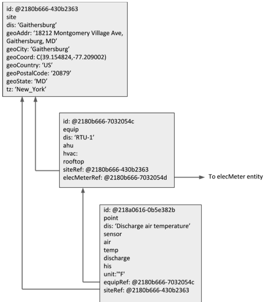
Figure 2.1: A Project Haystack sample project definition for a building in Gaithersburg Source: (Project Haystack, 2025a)
