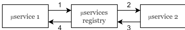
Figure 10: Server side service discovery. Service 1 asks Registry to fulfill the service (1,4); whereas Registry just proxies the communication to Service 2 (2,3).
