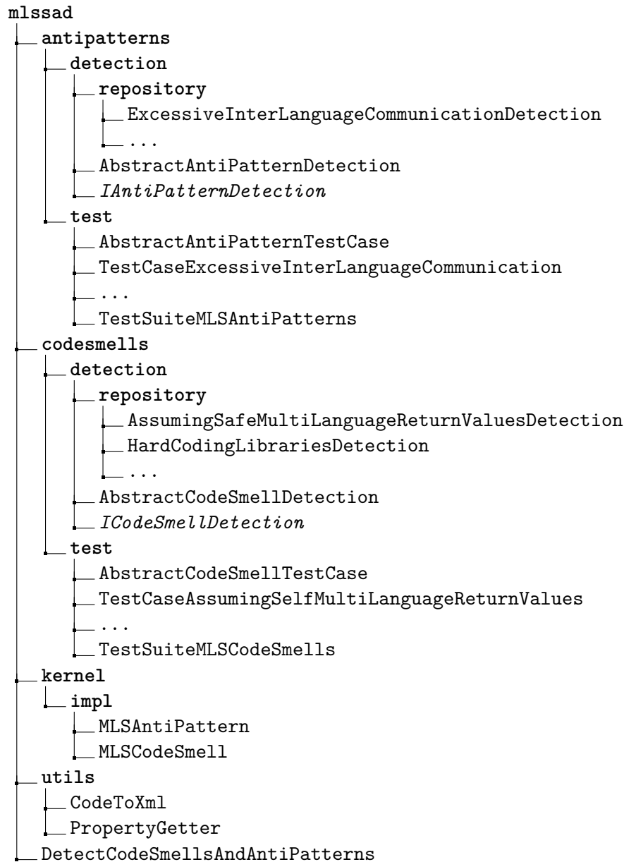
Figure 3: Directory tree of the mlssad package with packages , classes and interfaces
