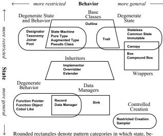
havior, or construction is degenerate, rectangles denote categories of patterns for containment, while trapezoids denote patterns used for inheritance.
